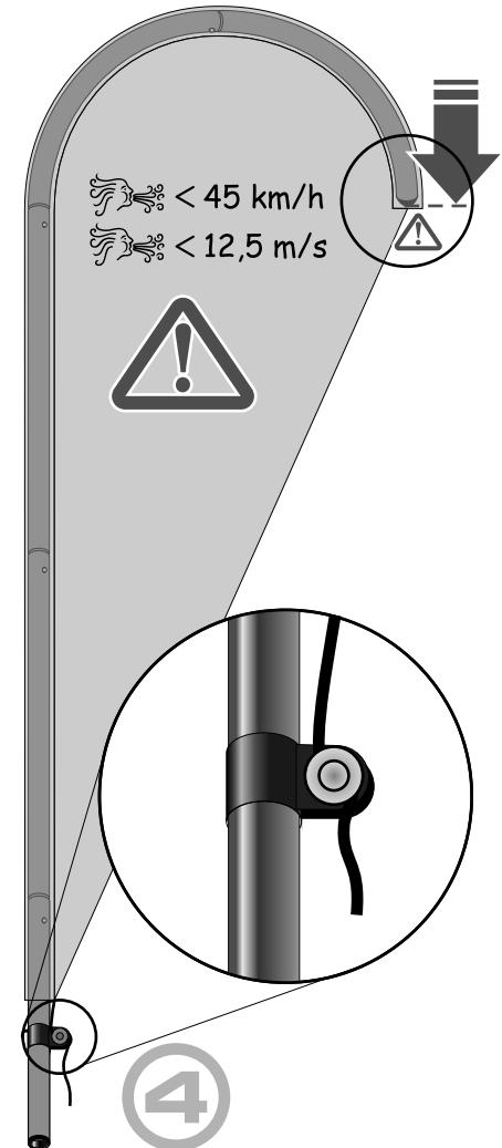
EN Ensure the tip of the pole reached the end of the flag sleeve.
